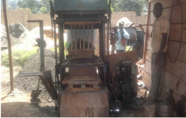
Concrete Block making machine and Blocks produced for the ongoing projects
